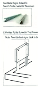
Two Metal Signs Bolted To Two C-Profile Metal Of Aluminum C-Profile To Be Buried In The Planter Note: Two identical signs back to back
